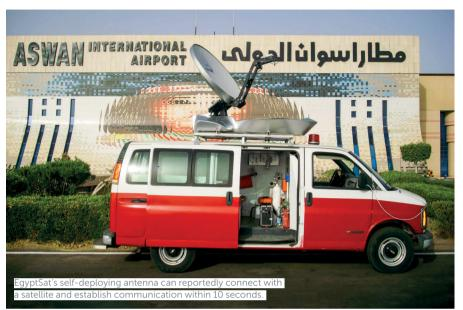
disaster area. Once the operator presses the button, it'll point the antenna to the satellite and establish communication within 10 seconds.
